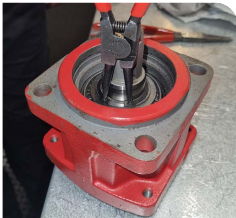
13. Disassemble the retaining ring (item 478)
