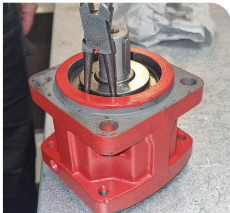
8. Disassemble the retaining ring (item 237)
