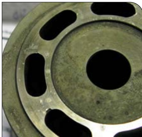
Cylinder barrel with severe damaged surface at the porting. The damage depends on contaminated oil due to poor filtration, clogged filter, previous break down or bad handling when filling the reservoir.
