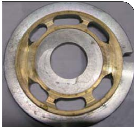
Valve plate with scratched surface.
