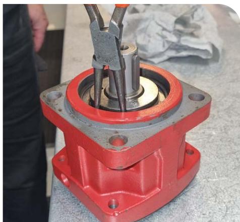
30. Install the retaining ring (item 237)
