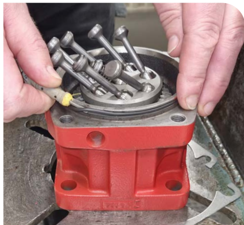
7. Remove the O-ring (item 221) Always change seal kit when removing seals
