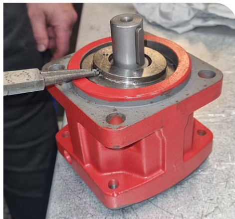
9. Remove the seal carrier (item 231)
