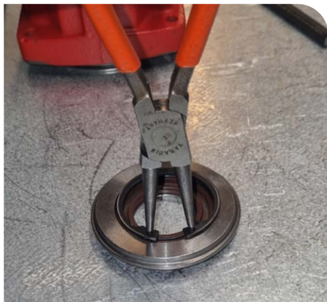
28. Assemble the retaining ring (item 238)
