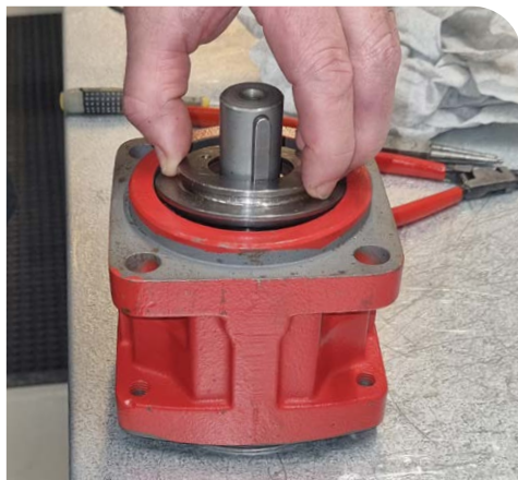
29. Install the seal carrier (item 231)
