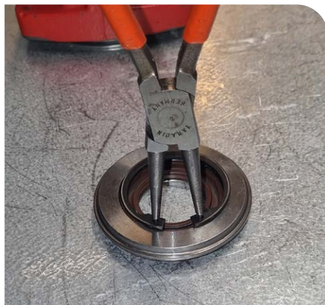
11. Disassemble the retaining ring (item 238)
