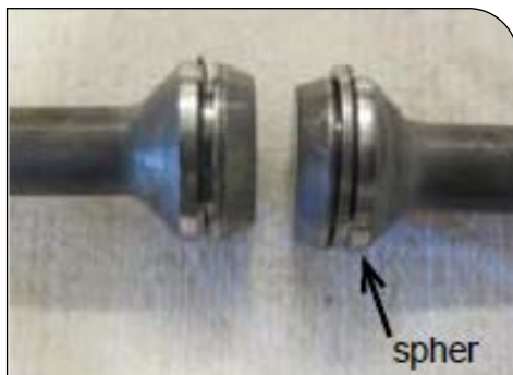
Pistons with worn out piston rings, some of them are missing and the spher is very damaged.
